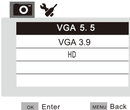
VGA5.5 ,3.9 and HD correspond to camera diameter 5.5mm, 3.9mm and 8mm respectively
